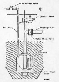
**Illustration 3** Liquid fills the ejector and discharge pipe until it starts filling the "U" tube from the discharge pipe. This stops air venting out the exhaust valve.
