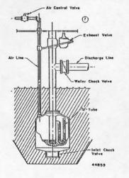
NOTE: The fill cycle of the ejector is very short (from 3 to 7 seconds depending on liquid level in well). The fill cycle is so short compared to the discharge cycle that for practical purposes the discharge is almost at a steady rate.
