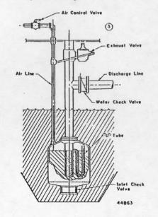
**Illustration 2 -** The liquid enters through the inlet check valve and fills the ejector.
