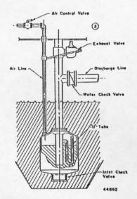
**Illustration 4** - Air pressure builds up over the liquid in the ejector, forcing it down and up out the discharge pipe. The level in the "U" tube follows the level in the ejector.
